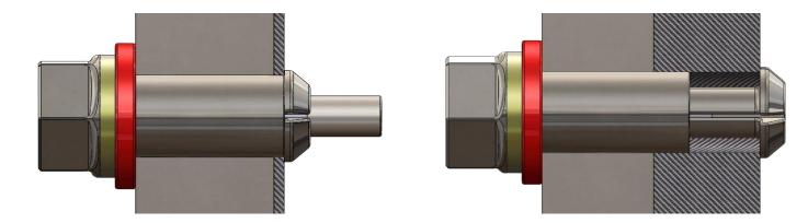
Our Hurricane design is focused on high load and larger hole size applications. The fastener uses an expanding petal design to enlarge on the blind side of a structure that pulls back on itself to provide clamping. The Hurricane Kwikbolt keeps holes true and provides a high clamp and high sheer performance. Head configurations include Flat Protruding (FP), Countersunk Protruding (SP) and Countersunk Flush (SF).
