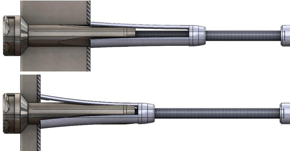
Our Storm design is focused on wet applications that require a low load and smaller hole size applications. The fastener uses a ‘clean and clamp’ process via an expanding leg design to enlarge on the blind size of a structure that pulls back over the main body to provide clamping. The Storm Kwikbolt keeps holes true, clean and provides a low clamp and high shear performance. Head configurations include Flat Protruding (FP), Countersunk Protruding (SP) and Countersunk Flush (SF).
